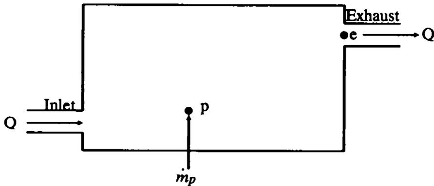
Fig. 7.1 Representation of a mechanically ventilated room.
