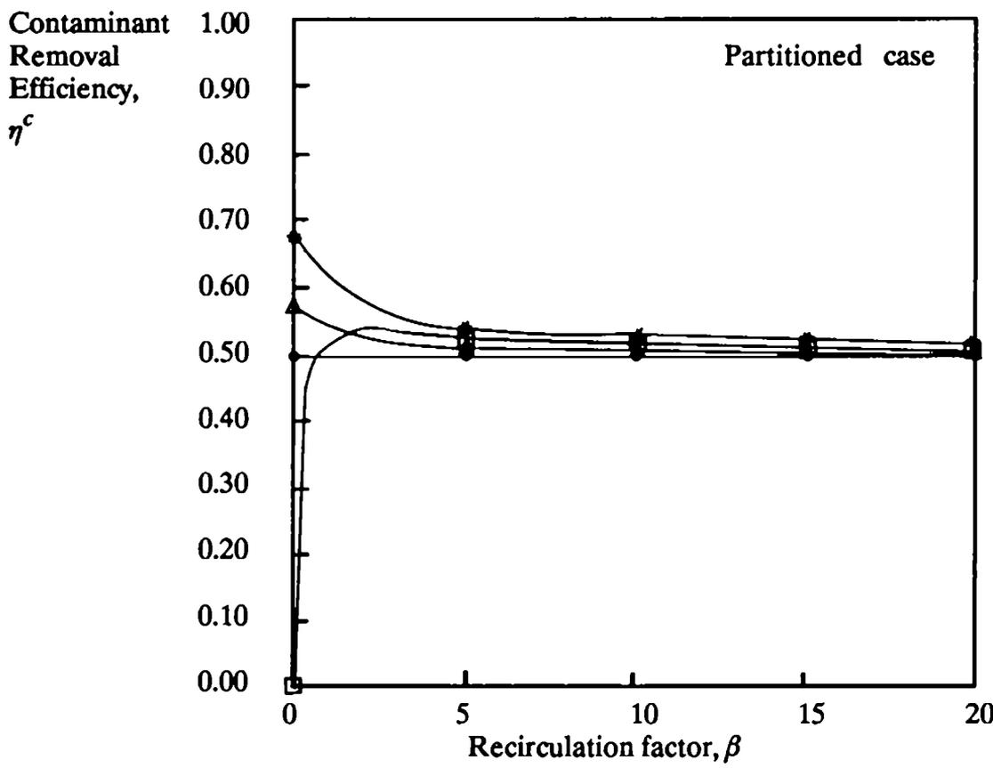
**Figure 5.3 - Contaminant Removal Efficiency vs recirculation factor.**
