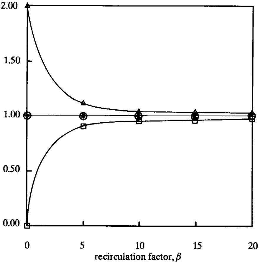
Figure 4.2 - Contaminant removal effectiveness vs recirculation factor.
