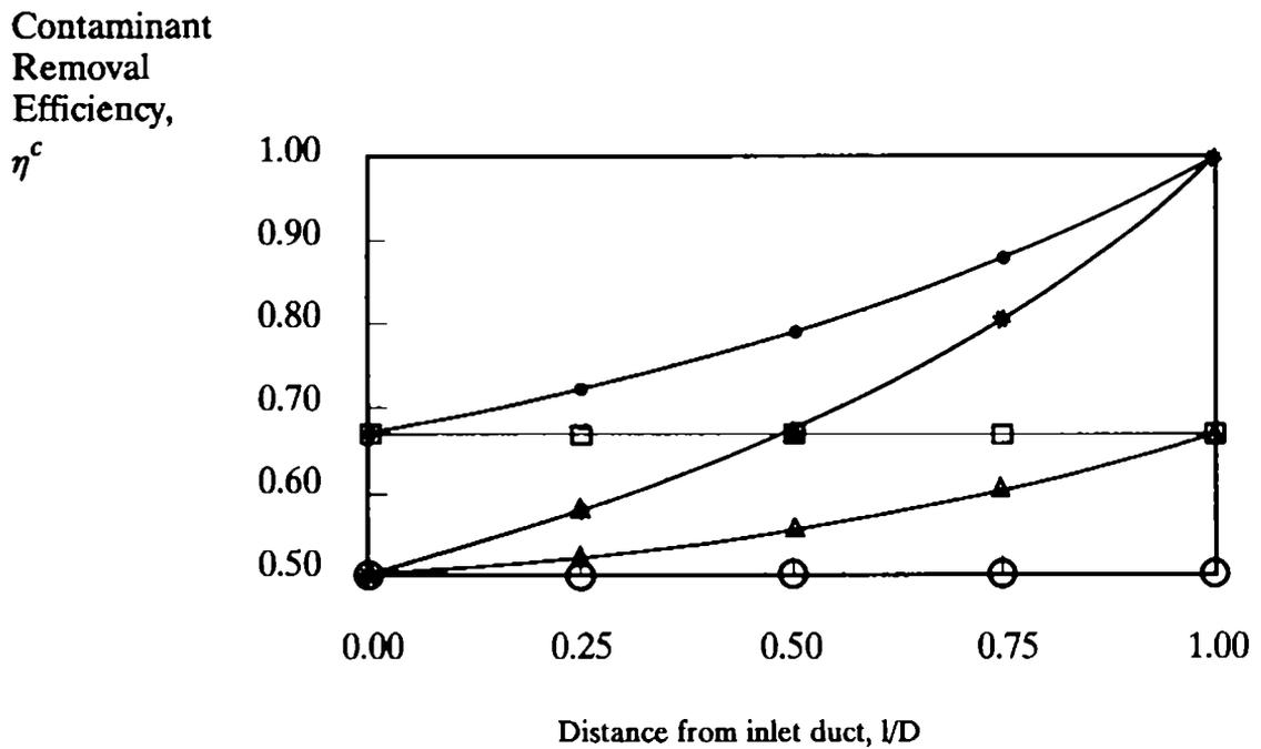
Figure 3.11 - Contaminant Removal Efficiency vs distance of contaminant source from inlet.
