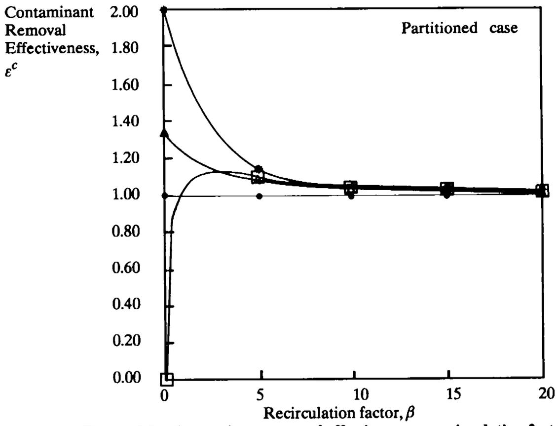
Figure 5.2 - Contaminant removal effectiveness vs recirculation factor.
