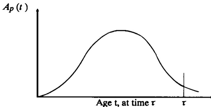
Fig. 7.2 Frequency distribution curve for the contaminant in the room.
