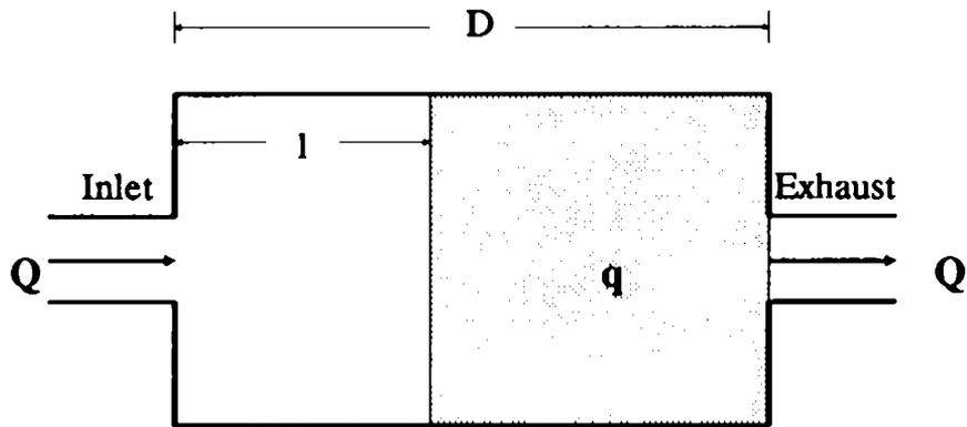
**Fig. 3.8 Piston Flow - Uniform Injection between a Plane across the Room and the Exhaust duct.**
