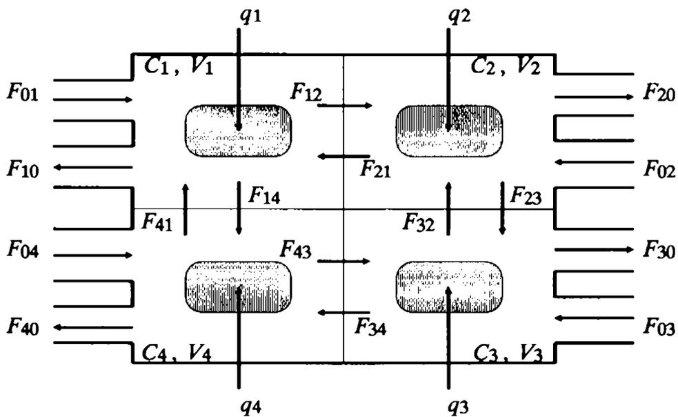
Fig. 5.1 Schematic Diagram of a 4 Zone Model
