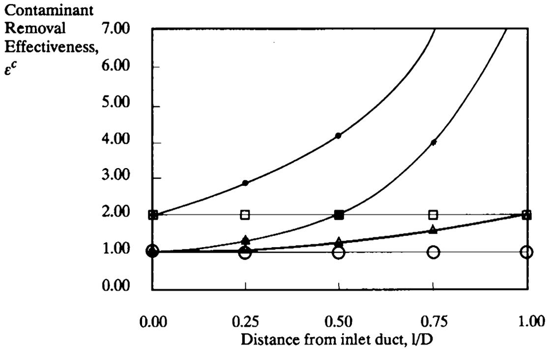
Figure 3.10 - Contaminant Removal Effectiveness vs distance of contaminant source from inlet.
