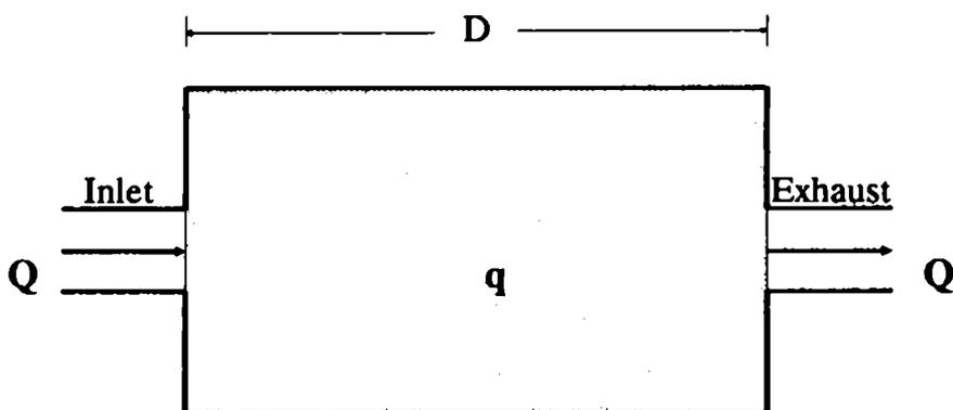
**Fig. 3.2 Piston Flow - Uniform Injection Throughout the Whole Space**
